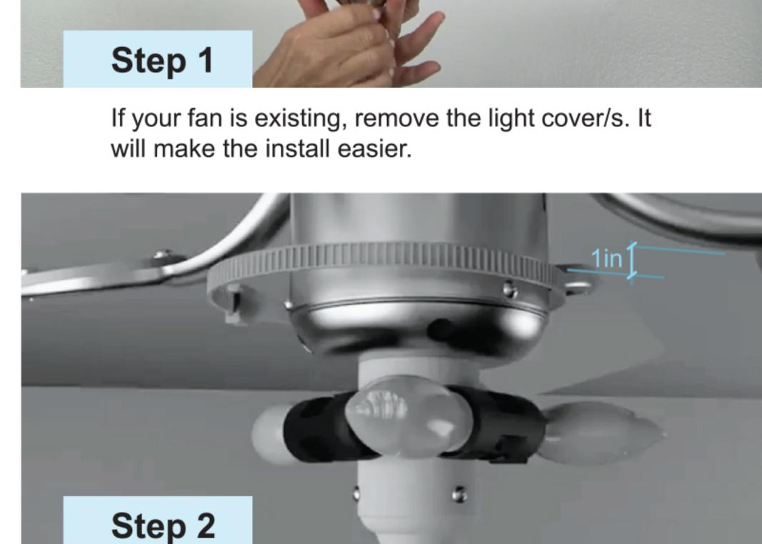
a flat space around the light housing at least 1 to 1 ½ inches below the fan blade.
